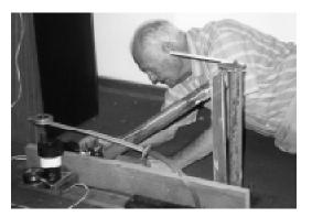
Figure 3. Danie making adjustments to his home-built seismograph. *AAVSO photo by Janet A. Mattei*.
