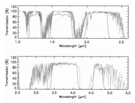
Figure 1. Atmospheric transmission from 1000 to 5500nm. Solid line is atmospheric transmission; dotted line is the filter response curves for the MKO filter system. From Tokunaga *et al.* (2002). *Copyright 2002, The Astronomical Society of the Pacific, reproduced with permission.*
