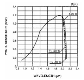
Figure 2. Spectral response curve for the Hammamatsu G5852 InGaAs PIN photodiode. *Courtesy Hammamatsu Corporation*.
