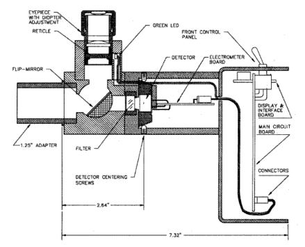
Figure 3. Cross-sectional view of the SSP-4. Courtesy of Optec Corp.
